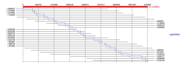
This diagram shows us that almost all of the reference genome is covered by tig00000001. However, most of these alignments are transpositions.
